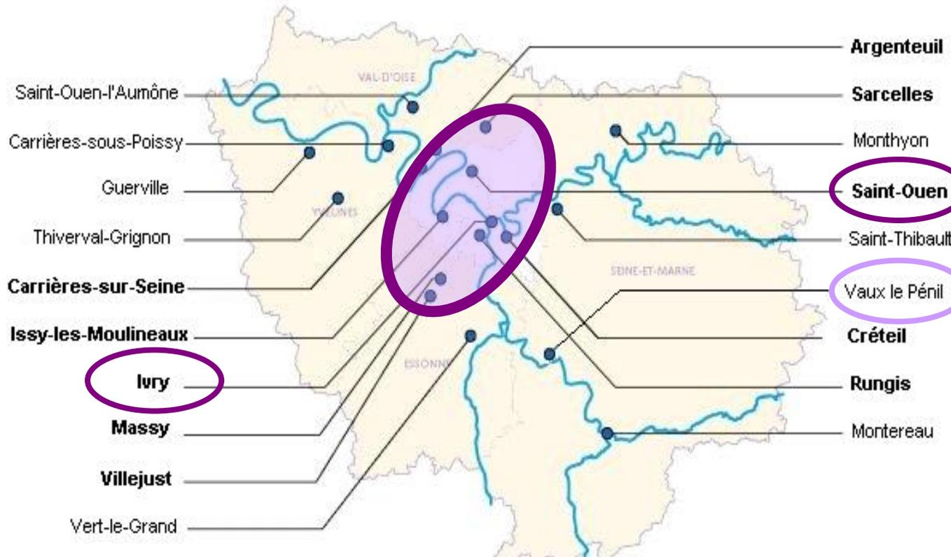
**10 EfW plants in the near suburb of Paris (70% of the IdF capacity) with NO<sub>x</sub> ELV down to 80 mg/Nm<sup>3</sup> instead of 200 mg/Nm<sup>3</sup> required by the directive.**
